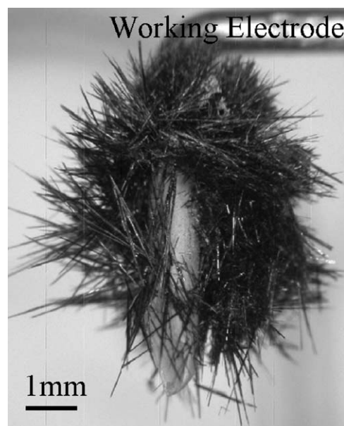
Fig. 3. Optical microscope image of crystals grown at the tip of the working electrode.
